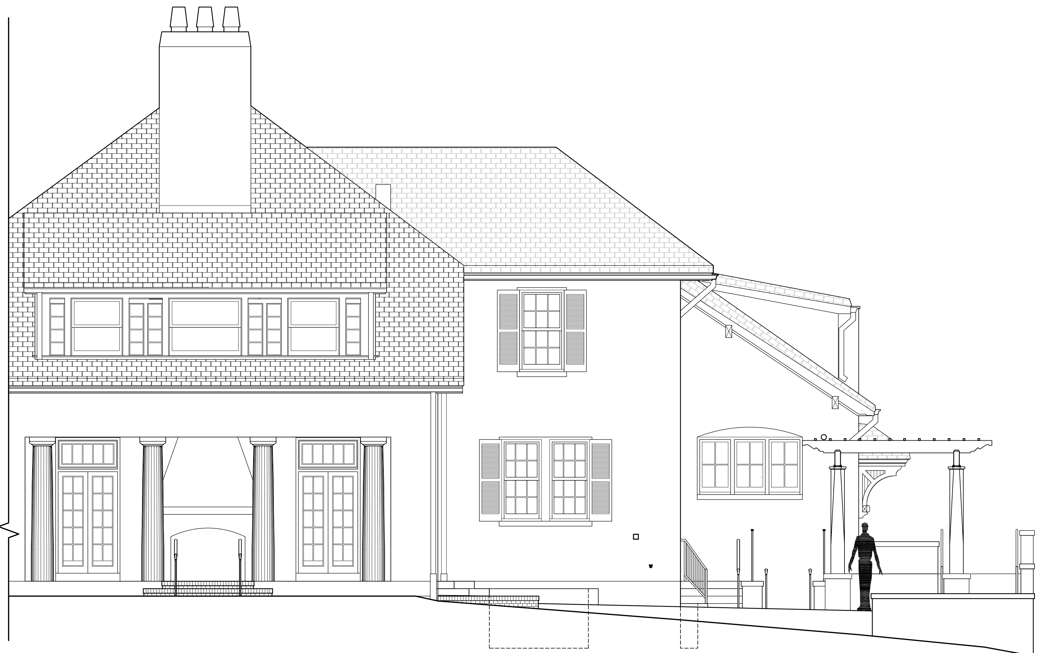
B2 PLAN EAST ELEVATION - OCTAGONAL TO SQUARE POST W/ STUCCO BASE & PRECAST CAP A1.0 | A2.1 SCALE: 1/4" = 1'
