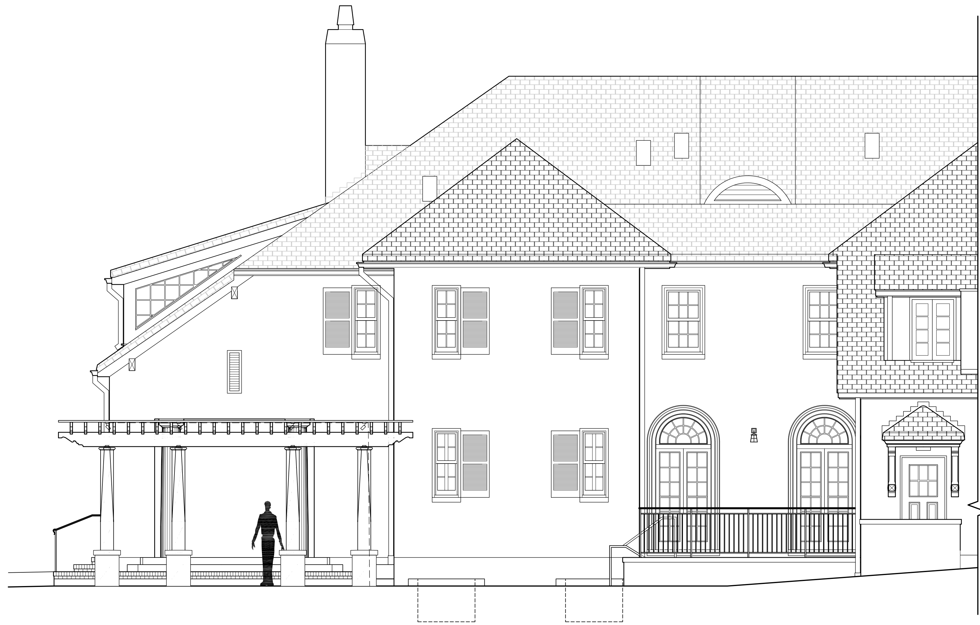
B1 REAR ELEVATION - OCTAGONAL TO SQUARE POST W/ STUCCO BASE & PRECAST CAP A1.0 | A2.0 SCALE: 1/4" = 1'
