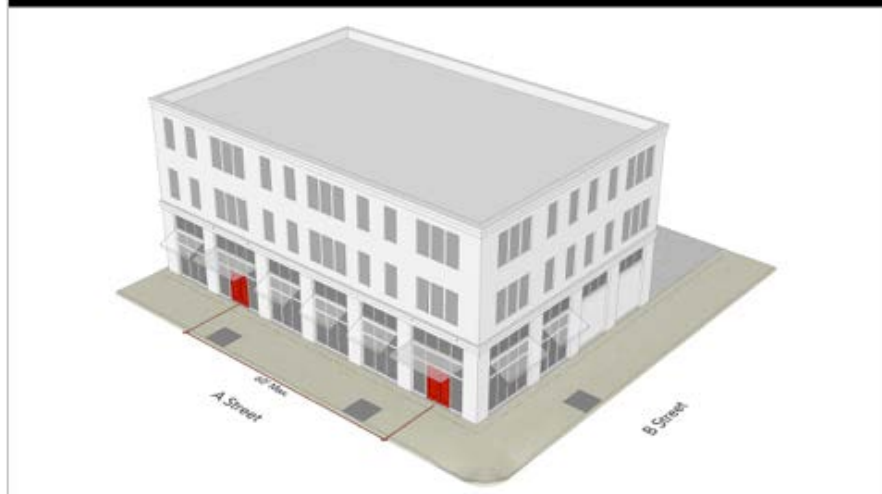
Figure 7.2 Frequency & Location of Doors on A & B-streets
