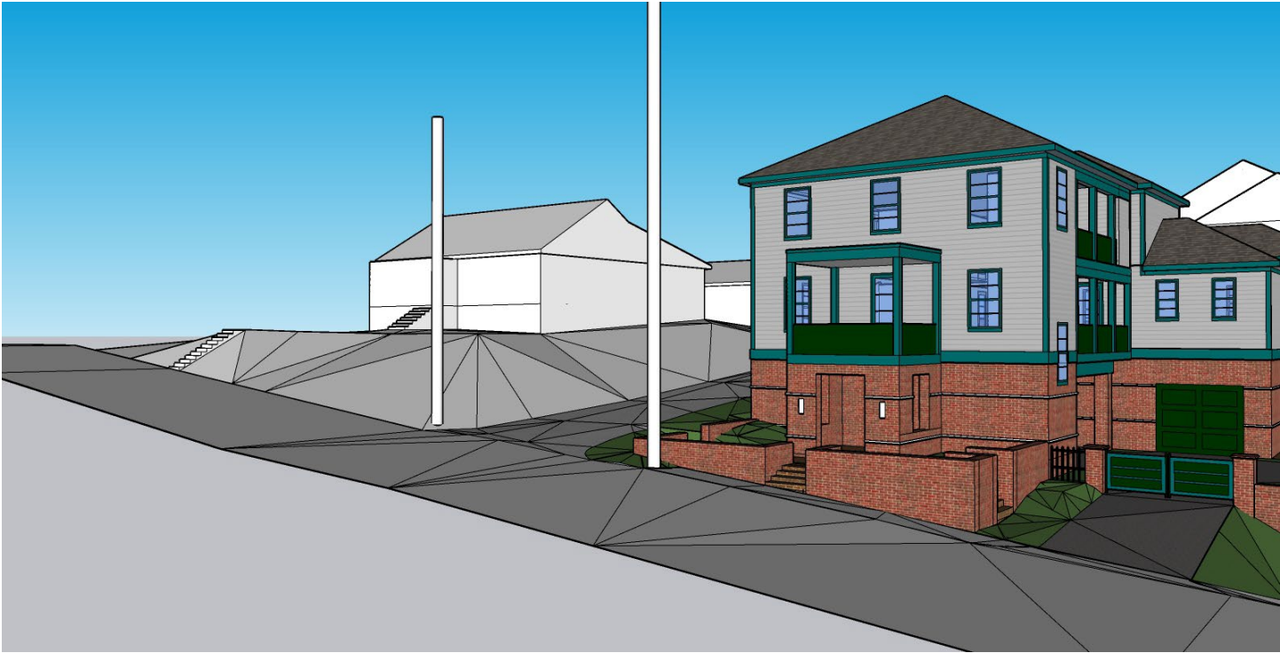
View of driveway & Scheme D ground floor entry with siding above brick foundation
