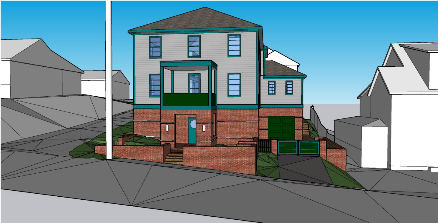
View of Scheme D ground floor entry, siding above brick foundation, solid gates at driveway and neighbor's fence beyond
