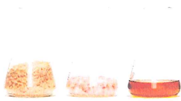
approx. 60% rice husks + approx. 22% rock salt + approx. 18% mineral oil = Resysta
