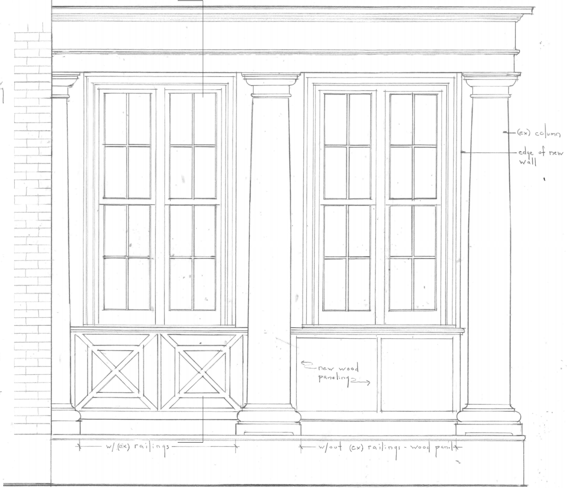
Enlarged Front Elevation @ north porch (typ) 3/4" = 1'-0"
