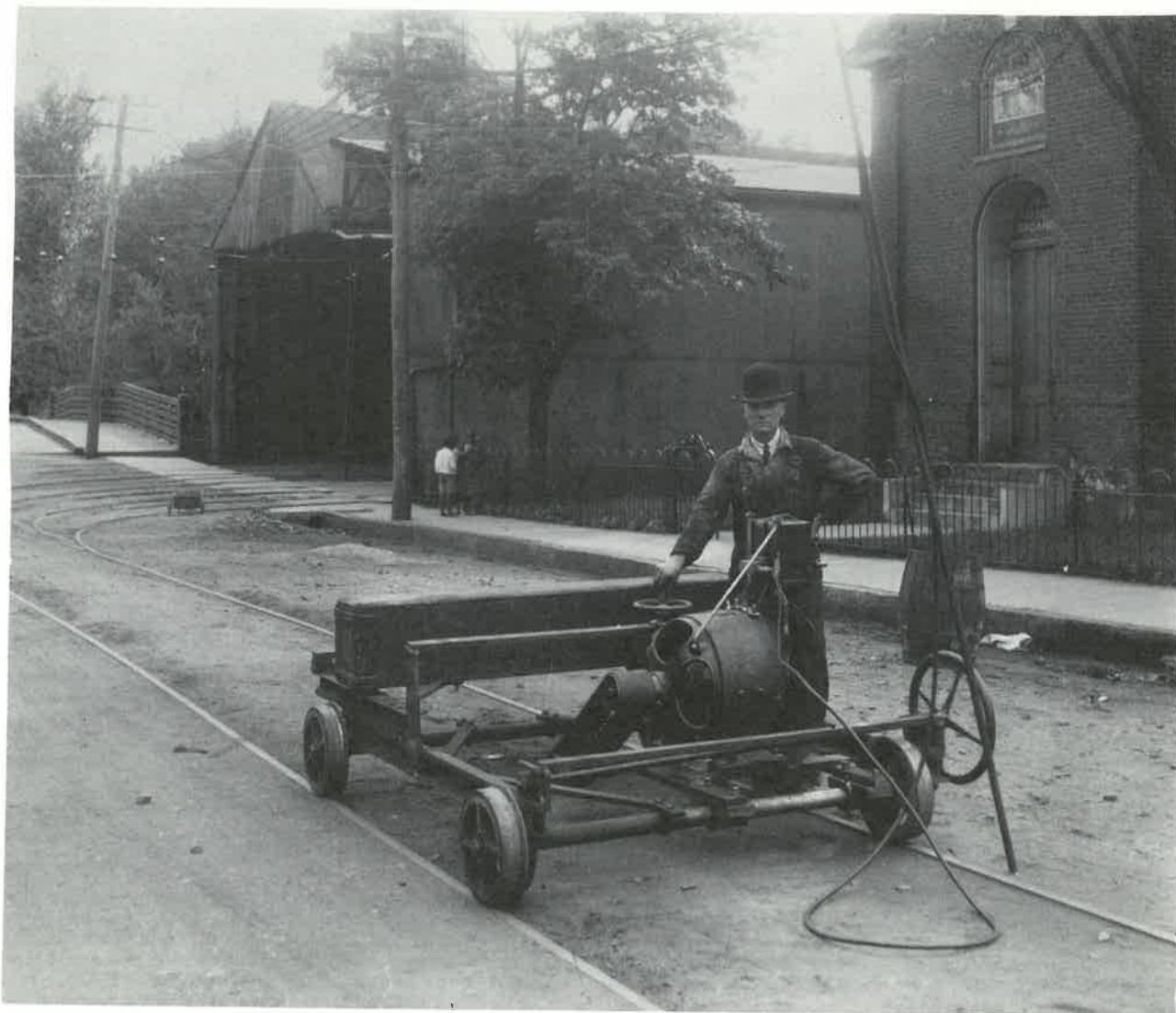
Superintendent Custis L. Carter and the rail grinding car he designed, May 1918. Note that a two-track leanto has been added to the original two-track car barn. Holsinger Studio Collection,
