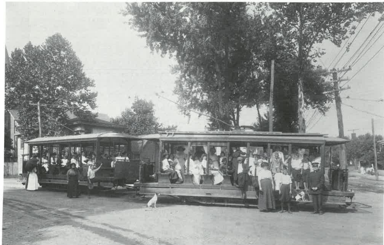
Cars 3 (at left) and 666 at Ridge and Main Streets on a Salvation Army outing on 14 August 1914. Car 666 was bought from Philadelphia in July 1912. The car roofs have been cut down in order to clear the C & O underpass. Holsinger.
