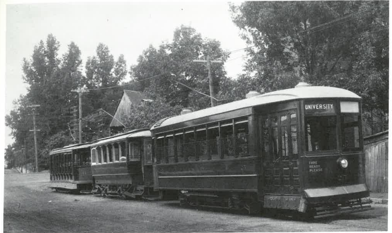
View south on Ridge St. showing from left, car 11, ex-Philadelphia Laclède, 4, built by Brill for Charlottesville in 1894, and Brill Nearside 25, taken 18 July 1914. The car barn is behind car 4. Note cut-down car roofs to clear C & O underpass. Holsinger.
