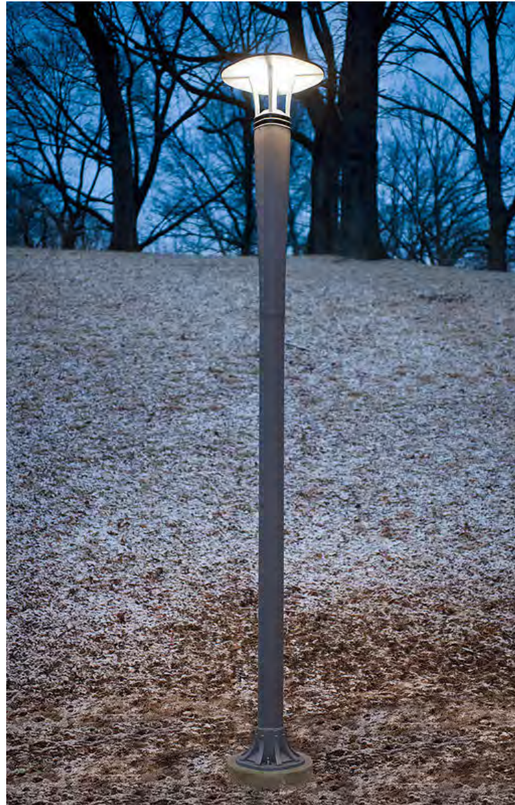
POLE LIGHTING TO REPLACE EXISTING CORDIA PEDESTRIAN LIGHTING - FORMS+SURFACES ALUMINUM, POWDER COAT FINISH DARK BRONZE METALLIC TEXTURE, 138" HEIGHT, 50W LED, 0-10V DIMMING CAPABILITIES, 3000K
