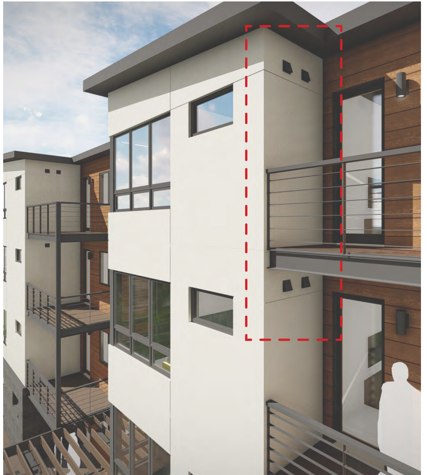
EXHAUST VENTS HAVE BEEN THOUGHTFULLY PLACED AND CONCEALED WHERE POSSIBLE. SEE A4.X SERIES FOR MECHANICAL DIAGRAMS AND 2.X SERIES FOR EXTERIOR ELEVATIONS
