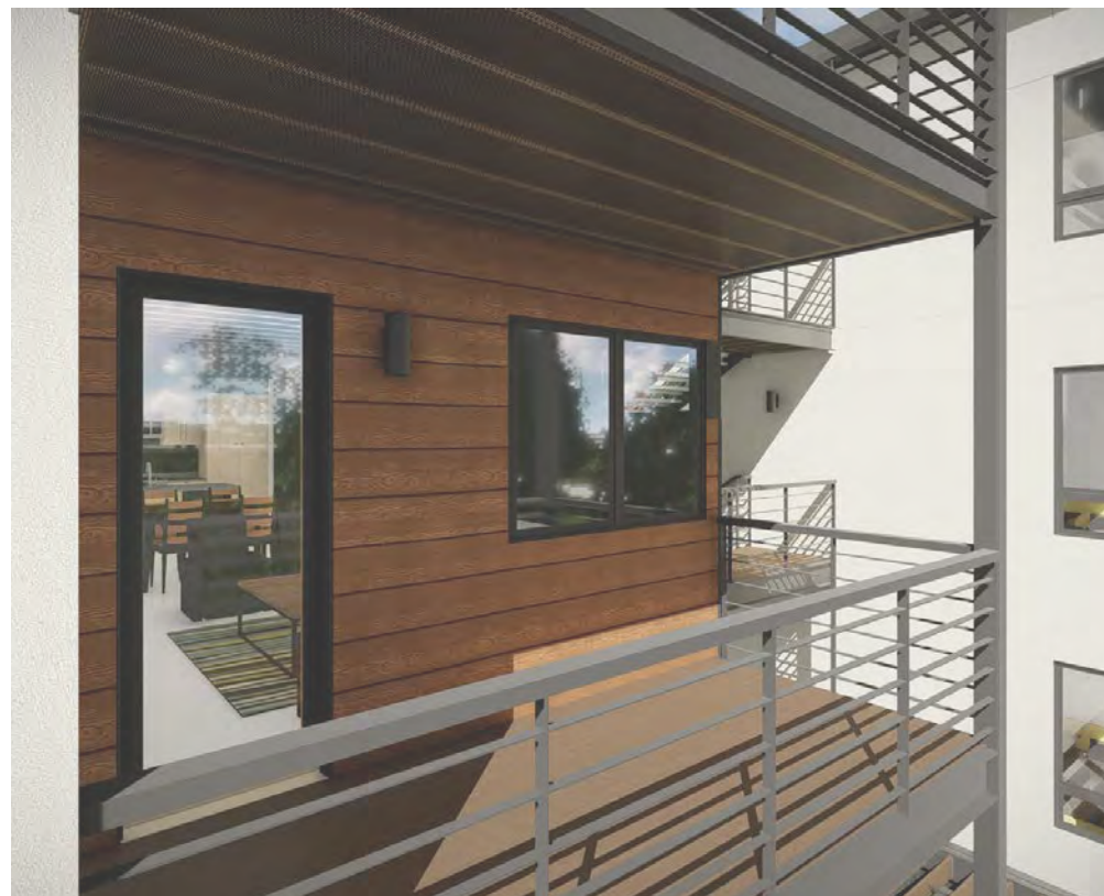
LAP SIDING AT DECK
