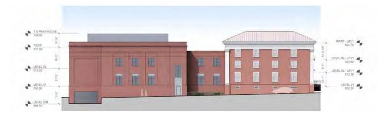
This adjustment brings down the scale fronting the Jessup House. The north elevation is proportional to the Levy Building expressing the chambers within and sets back from Levy. The lowered hyphen restores the full historic cornice of Levy along the east side. Stairs on the north and south are expressed in an adjustment to fenestration heights and further breaks the scale down for the neighboring streets.
