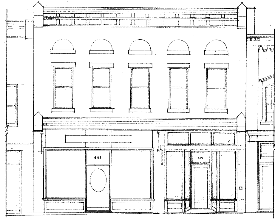
1 BUILDING ELEVATION - EXISTING CONDITIONS W/ PROPOSED FACADE 1/4" = 1'-0" (FULL SHEET SIZE) 1/8" = 1'-0" (c 50% REDUCTION)
