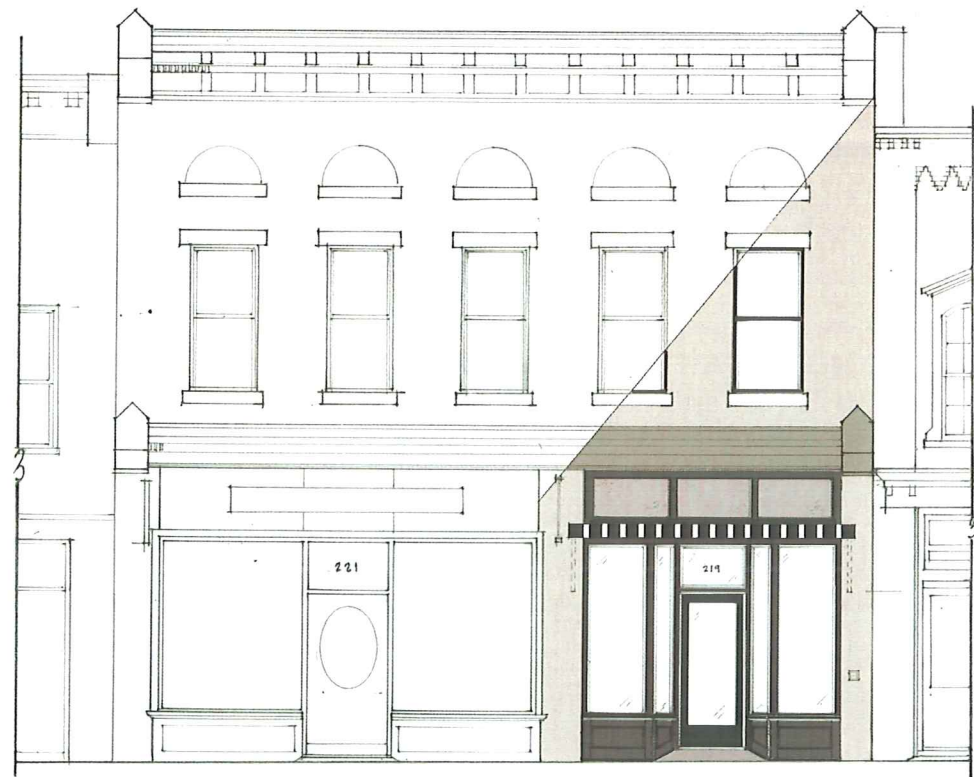
1 BUILDING ELEVATION (See Sheet A2 for scaled drawings) P4 Proposed based on a 1921 Facade Design
