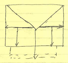
basic form; med his uf steep gables centered on each side a over side bays of facade, plus steeper & somewhat taller gable in center of facade as extending out over porch roof
