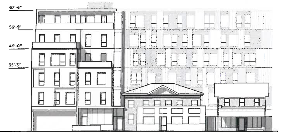
510-600 W. Main Street 67'-6" + Appurtenance 4 stories: 24' setback from face of curb story 5: 12'-6" stepback story 6: 6'-6" stepback sidewalk width: 8'
