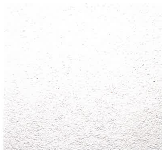
NEW STUCCO -FINE SAND FLOAT FINISH
