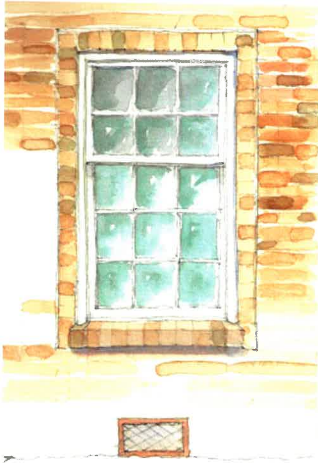
Window detail (not showing bars.) Note brick reveal surround.
