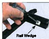
Tightening rail wedge on shortened section.
