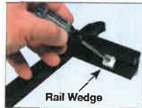
Tightening rail wedge on shortened section.
