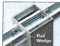
View of the underside of bottom rail to show rail wedge location.
