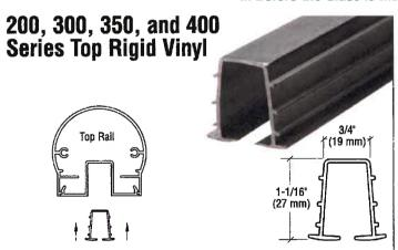
CRL 200, 300, 350, and 400 Series Top Rigid Vinvi is available in two sizes to hold 1/4" or 3/8" (6 or 10 mm) glass. When installing Rigid Vinyl, snap it into place before installing the glass. Stock lengths are 12' (3.66 m).
