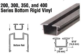
CRL 200, 300, 350, and 400 Series Bottom Rigid Vinyl comes in two sizes to hold 1/4" or 3/8" (6 or 10 mm) glass. When installing Rigid Vinyl, snap it into place before you install the glass. Stock lengths are 12' (3.66 m).
