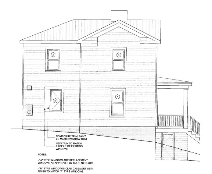
ELEVATION - NORTH SCALE: 1/4" = 1'-0"
