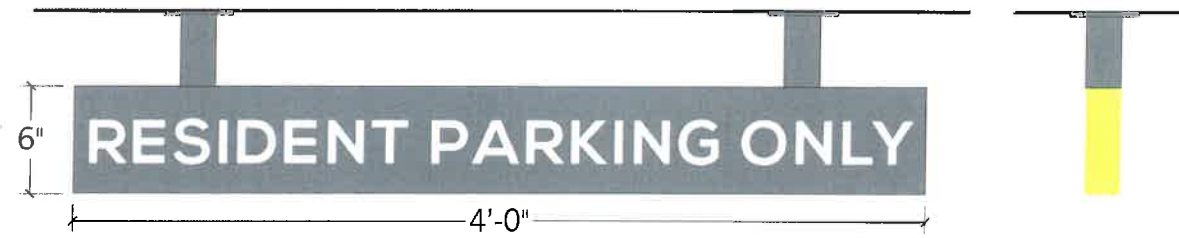
2 Front/Side Elevation HANGING SIGN, H1 (OPT 1) Scale: 1" = 10" ALUMINUM CABINET W/ PAINTED AND REFLECTIVE WHITE VINYL DECORATION
