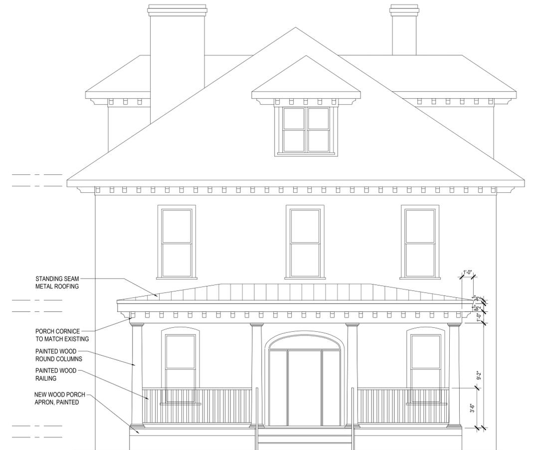
**EXTERIOR ELEVATION - NORTH ELEVATION**
