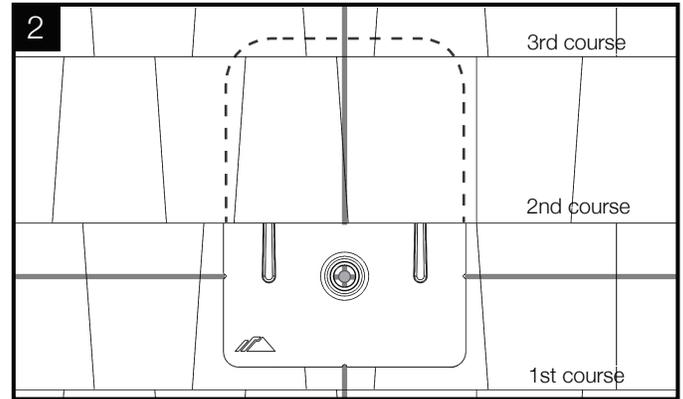
Slide flashing between 1st and 2nd course, so the top is at least 3/4" above the edge of the 3rd course and the bottom is above the edge of the 1st course. Line up pilot hole with view port.
