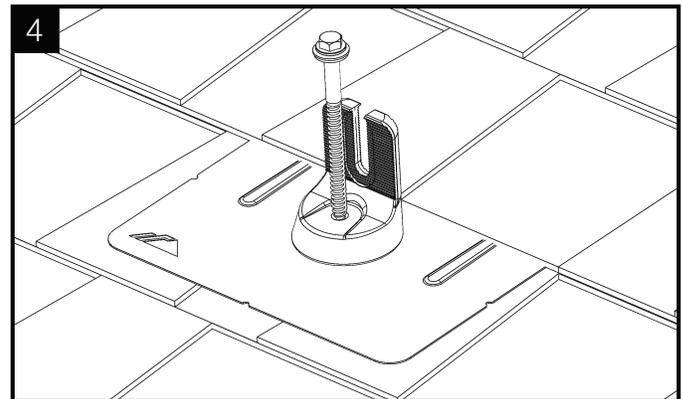
Insert lag bolt with EPDM backed washer through flashing. Tighten lag bolt until fully seated. FlashVue is now installed and ready for IronRidge XR Rails.
