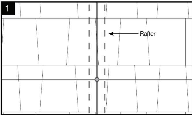
Locate rafters and snap vertical and horizontal lines to mark locations of flashings. Drill 1/4" pilot holes, then fill with roofing manufacturer's approved sealant.
