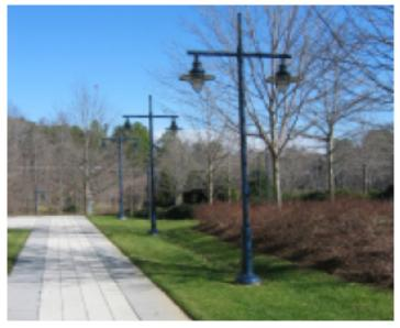
Shielded lighting mounted on pedestrian-scaled poles focuses light on where it it needed - the sidewalk.
