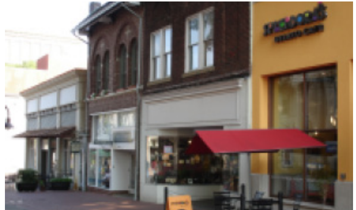
When renovating or designing a new storefront, consider using a traditional three-part facade of cornice, upper story windows and a storefront with an articulated base.
