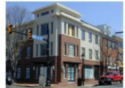
This corner infill building uses a change in materials to reduce its mass.
