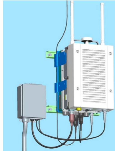
Antenna/equipment cabinet micro design
